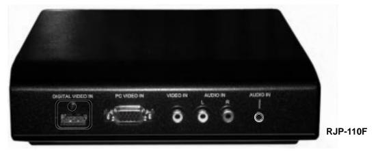
The Remote Jack Pack (RJP) contains circuitry to determine the presence of a signal at each input jack.
